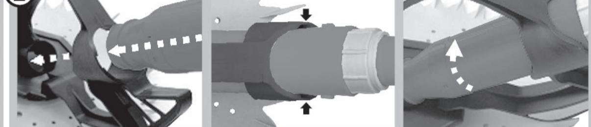
GB Insert the diaphragm chamber "C" into the support "A". Align the side pins on diaphragm chamber with the notches on the support "A", and continue to insert the chamber into the chamfer of the support. Follow the arrow direction of marking "O" and turn the chamber until it stops.
