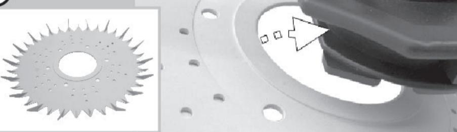
GB Place the mat "E" under the cleaner support "A" and make sure the fins are pointing upwards. Start by inserting the inner edge of the mat into the front groove of the foot pad "B". Stretch and insert the mat all around the groove. The mat should be secured in the groove and free to rotate on the foot pad.
