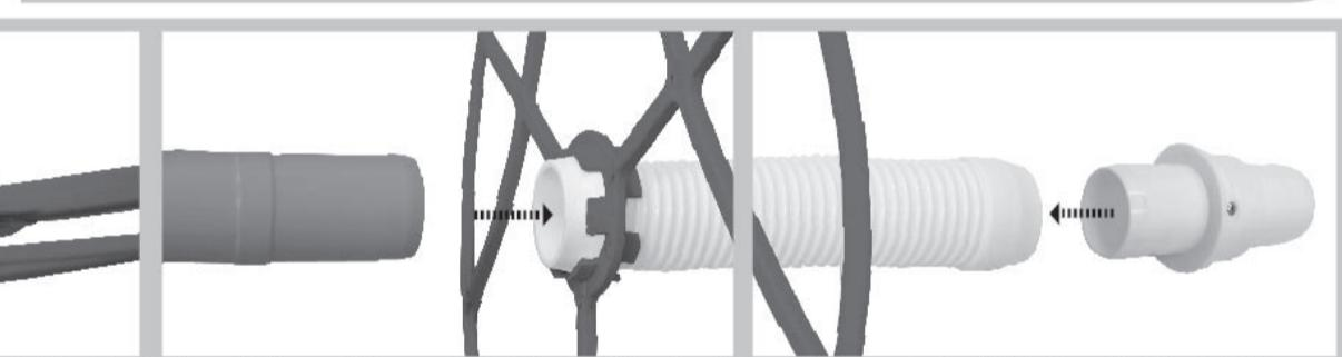
GB Place the top ring "R" on a flat surface with its marking "TOP" facing upward. Insert either end of hose "K" into the central hole of the top ring until its hose cuff is secured by the tabs. Insert the cuff on the top of diaphragm chamber "C" into the end (with top ring) of hose "K" as far as it can go. Insert one side of swivel connector "F" as shown into the other open end of hose "K" as far as it can go.
