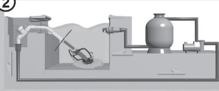
**GB** To connect your cleaner to your skimmer, remove the basket and vacuum plate, and insert vacuum plug "I" into the hole. Assemble the elbows "H" on both ends of pressure regulator "J". Follow the arrow marking on the pressure regulator to connect the corresponding elbow to the vacuum plug and then connect the other elbow with hose "L" as shown.
