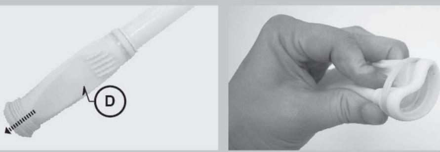
**GB** Pull out the diaphragm from the connection tube. Squeeze the diaphragm a bit and then take out the retaining ring. Now you can clear the inside of the diaphragm and connection tube. **Notice:** Never put sharp objects inside diaphragm which may damage it and then affect the cleaning function. After clearing the diaphragm and connection tube, reverse the steps to assemble back the diaphragm chamber. Make sure the retaining ring is on the diaphragm.
