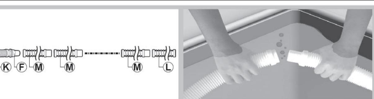
GB First, lay down all hose sections on the ground under sunlight for about an hour to remove hose memory. Second, measure your pool to figure out total length of hose needed for cleaner operation. Total length of hose after assembly should be half to one hose section length longer than the length measured from pool skimmer / dedicated suction line to the farthest point in the pool.
