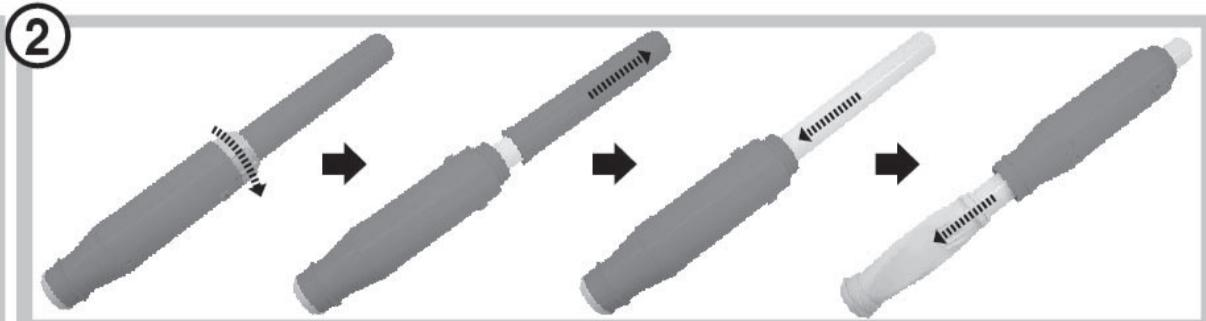
GB Follow arrow direction of marking "O" to turn the diaphragm chamber to release it from locking position. Remove it from the support "A".
